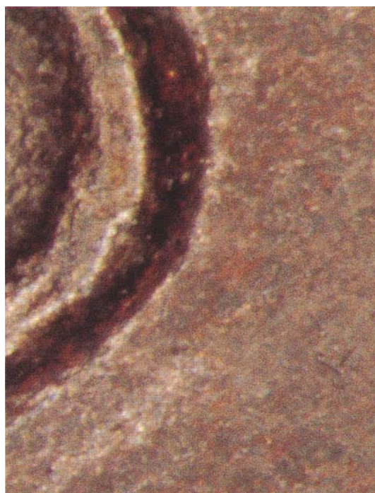
2. Photomicrograph, fig. 9, obverse, showing granular characteristics consistent with sand casting. View shown is upper left area
