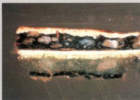
Photomicrograph of cross section A, view 2: sample in cross section A, stained with amido black 3 (110x)
